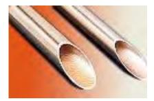
(2) <u>Multi-Grooved Tube</u>: A seamless copper tube with a smooth outer wall and grooves cut into the inner wall. The grooves increase the inner surface area, dramatically improving heat transfer efficieny. Compared to the efficiency requirements of smooth tubes, it reduces the amount of copper tubes used in the heat exchanger production process. It is therefore utilized to produce highly efficient and expensive small-type air conditioners.
